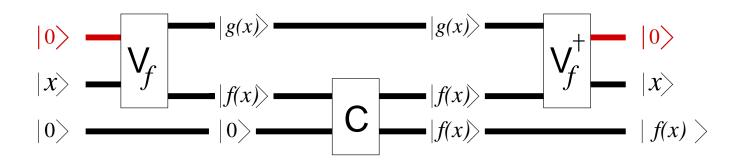
${f C}$  is built out of 1-Qbit controlled-NOT gates:
